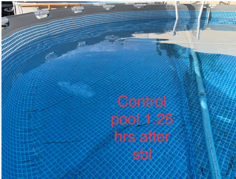
Figure 7 – Control Pool After 1.25 hrs of Introducing the Bather Load – Material Still Floating
